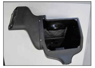
8. Install the AIRAID® fresh air intake into the AIRAID air filter housing and secure with the provided hardware.
