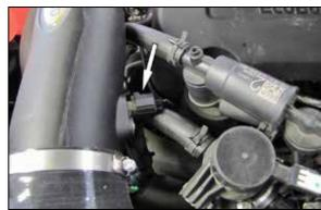
22. Using the provided extension harness, reconnect the inlet air temperature sensor.
