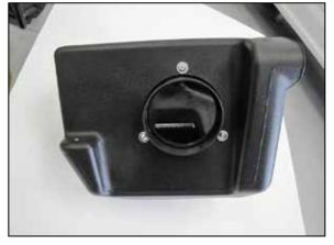
6. Install the filter adapter into the AIRAID® filter housing and secure with the provided 1/4" hardware.
