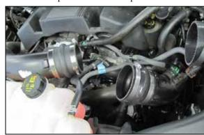
17. Install the two remaining coupler hoses onto the turbo inlet tubes and secure with the provided hose clamps.
